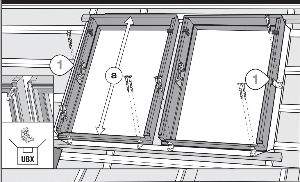
ENGLISH: Install windows ensuring that the window bottom frames are flush. Adjust windows (see instructions enclosed with the windows). If adjustment is required of the frame sides facing the UBR, adjust the UBR brackets (1). Then fit the underfelt (see instructions enclosed with the windows) and the flashing (see instructions enclosed with the flashing).
