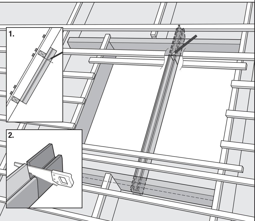
ENGLISH: Adjust UBR at the ends. The measurement X must be maximum 40 mm when cutting out the UBR.
