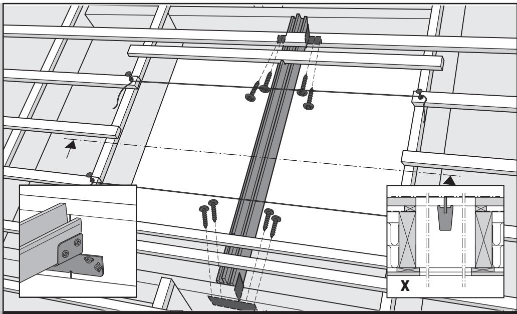
ENGLISH: Fit seals supplied into the two window rebates to be positioned onto the UBR (1). Fix brackets supplied with the windows to the frame sides opposite the UBR (a). Fix brackets supplied with the flashing to the frame sides facing the UBR (b, c).
